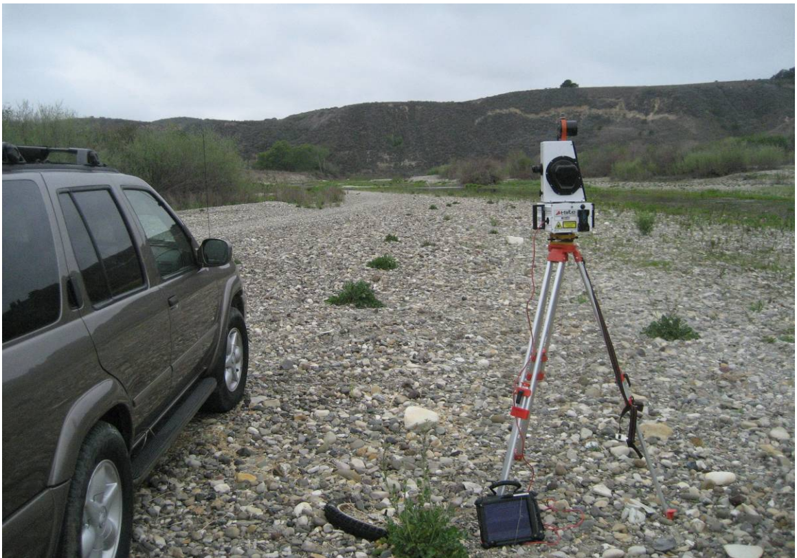
Figure 41: Pre-project Terrestrial LiDAR survey
