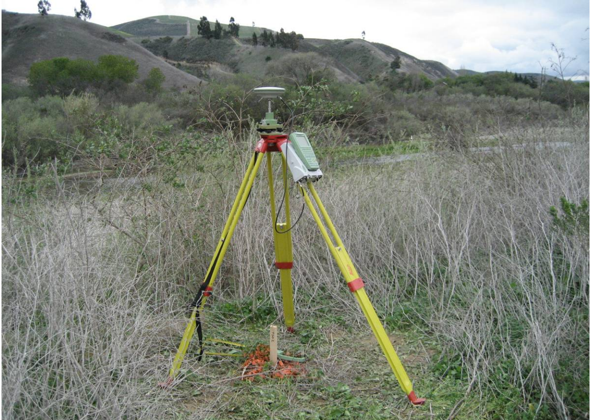
Figure 42: Survey control was established to allow for georeferenced surveys.
